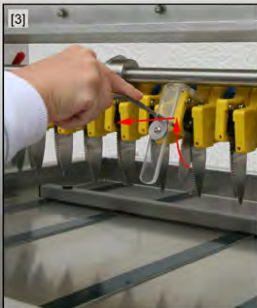
[3] + [4] Blade-click system for quick removal of blades
