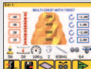
Each layer of the tower can be deposited in alternate clockwise and anti-clockwise directions
