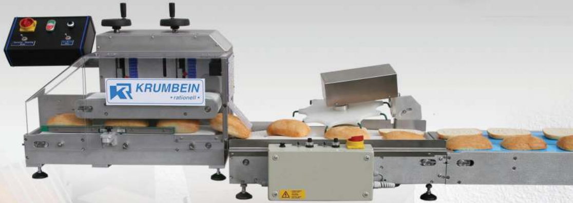
Splitting device in combination with BBS VE and covering conveyor
